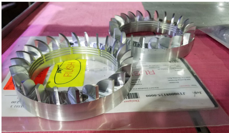
Figure 4: Redesigned front wheel seals
